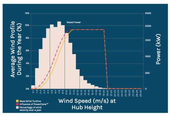
The baseline power curve and wind speed distribution seen here comes from a generic 2MW turbine located in an IEC Class IIa wind regime, and is reflective of expected power gains.
